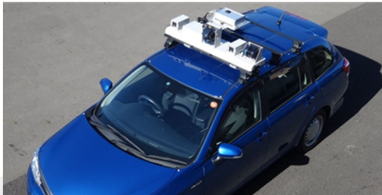
Road Surface Properties Measuring Vehicle
