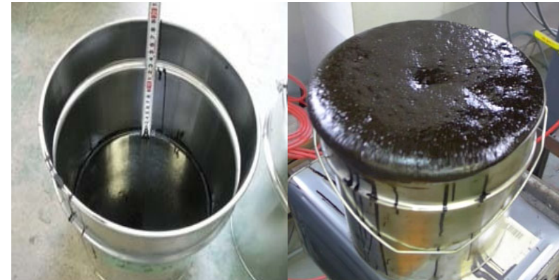
Mible-eco (generic term: foamed asphalt mixture)
